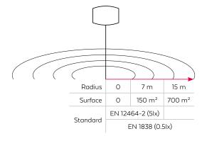
How to read the drawing: in a range of 15 m, being a surface of 700 m², we guarantee a lighting in accordance with the EN1838 standard.
